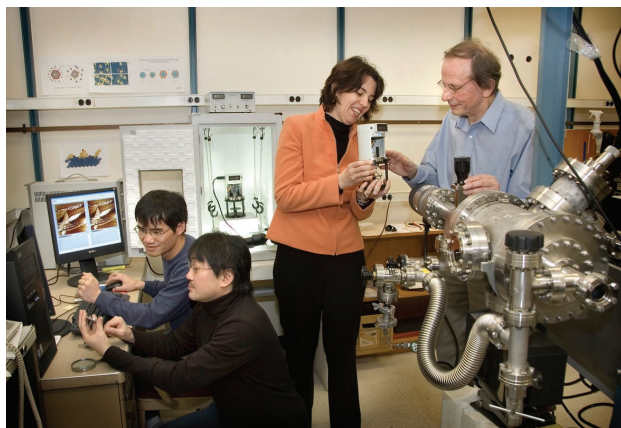
(Clockwise) Brookhaven Lab researchers Kotaro Sasaki, Junliang Zhang, Eli Sutter and Radoslav Adzic view gold clusters on a single-crystal platinum surface using a scanning tunneling microscope.
